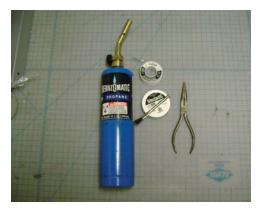
The tools you'll need are; A propane soldering set Water-based paste flux and brush Lead-free plumbing solder Needle-nose pliers
