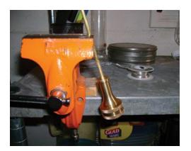
Apply the paste flux to both parts and fit together. Hang by gently clamping the tubing in a vice, or have a helper hold it with a pair of pliers (it will get hot).
