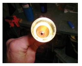
If you get a small amount of solder drip in the nozzle you can file it, or just leave it- the whole point is flow restriction anyway. Now re-insert the rubber washer.
