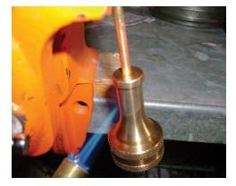
Heat the nozzle with the propane torch, this will facilitate a better flow of solder.
