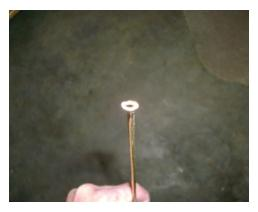
Take the needle-nose pliers and gently flatten and pinch the end of the nozzle- this will give you a good sweep area and increases the pressure. Heck it did a great job on my basement floors! The final step is to check your work- hook it up to a garden hose or sink with garden hose threads, plug the tip with your finger, turn on the water and see if the soldered joint leaks.
