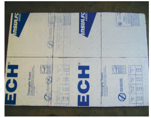
This is a 4' x 32" sheet of 1" thick styro insulation, marked in 16" squares, you can get 4 lids out of 1 4'x8' sheet. 16" fits perfectly on the cooler.
