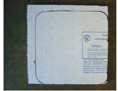
Here's the lid outline, this will rest inside the cooler creating the seal. Cut just inside your marked line.
