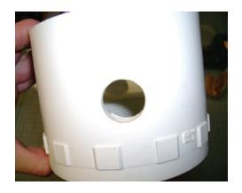
Using a 7/8" drill (this holds the PVC tube very well), drill both sides and give it a light sanding or filing to remove the burrs.
