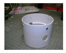
Here's the coupler fitted with screws and both holes drilled. I used the shortest pan-head machine screws I could find, and ground the points down with a dremmel tool after I installed.
