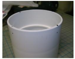
Alternately, you can a use cheaper 4" straight PVC coupler and just mount some screws to hold up the clamp (only about \$1.25 at Home Depot). I've marked for 4 screws here. Drill a small pilot hole for the screws to make it easier to install them.
