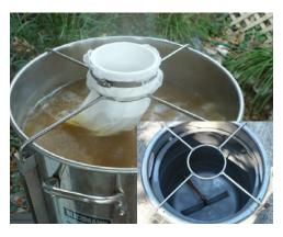
Here's a fancy one. All welded and a 4" to 3" reducer coupler rests on top.
