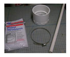
Here's all the parts, 4" PVC coupler, a hose clamp large enough to fit around it, a length of 1/2" PVC tubing and 5-gallon paint straining bags. The paint bags are a finer mesh than a large nylon 'grain bag'. I picked up this coupler as it had a ridge to hold up the clamp. It cost about \$4 at OSH.
