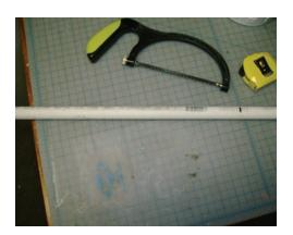
Measure and cut the PVC to your needed length. If you have a standard kettle, be sure to have an extra 3-4" on both ends beyond the kettle diameter. If you have a keggle, check the fit and cut more if necessary.
