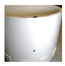
Mark down both sides for you drill center point. Be sure to leave enough room above the ridge for the hose clamp.
