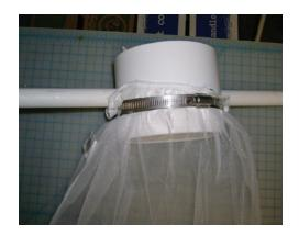
This is how it all goes together. On this one, I didn't account for as much space above the clamp as I'd like for the support bar, but it still fits fine, just snug. You can also put in a screw on one side of the tubing so the coupler won't slide when you lift it up.
