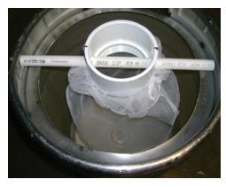
So here's how it'll sit in the keggle. Make sure you've pulled up enough of the paint bag so it won't be on the bottom and melt or scorch. Throw your hops right in, and just lift it out when you add the immersion chiller, and put 'er right back.
