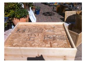
If I had cut the entire side to fit and then cut the two pieces apart, it would leave a 1/8<sup>th</sup> an inch gap between the two boards because of the wood lost to the saw blade. I cut the final piece and made all the pieces fit snugly. It looked good, so I drilled and cut the hole for the tap line in the tower.
