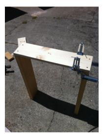
If I were buying all the lumber anyway, I'd have bought the same dimension because it saves a step. The board width will be determined by the internal height you need. With my fridge I needed about 3 inches of additional height to allow for a 5 gallon fermentor and airlock. There will be an additional 2 inches used by the top, so I had to go with at least 5 inches of collar height.
