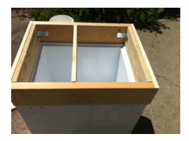
Next I cut another piece of 1x6 to go in the middle as a brace. I then placed the collar on the ground and placed a corny keg inside and the lid to my 5 gallon bucket inside. I used this to guide where I was putting my brace. I already knew it was a close fit, but this way I couldn't screw up the measurement. I placed the centerboard accordingly, and screwed it in. I tossed it back on and to reassure myself I slid in my keg and bucket. All was well.
