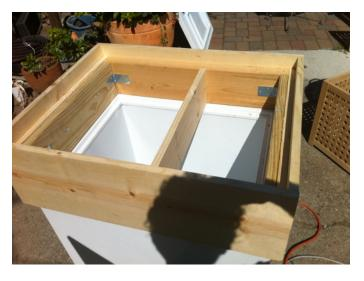
Now when the collar goes on top of the freezer the 1x10's will hang over the top of the freezer by 2 inches and prevent the collar from shifting in any direction. They will also be above the 2x6 collar by around 2 inches. This will provide what will hold the top pieces in place.
