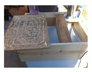
Since I was using nice wood on top of ugly wood, I cut and glued the finishing pieces. I left my finishing pieces a little larger than the base piece, and sanded them down. This way there are no gaps on the top.
