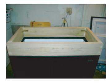
Here's the drilled and fitted top. joints are glued and attatched w/3" counter-sunk screws (you can see the wood filler in the holes and between the joints)
