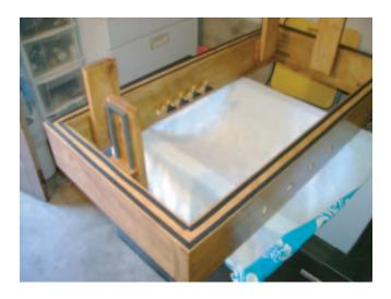
Here's what it looks like w/ the braces installed. i applied some rubber window stripping, I think it was 3/16" thick and 1/4" wide. I also laid a thick bead of clear silicone II sealant between the foam just before final install after all the fitchecks. I used some foam stripping on the braces to make sure I got a snug fit. Mount them, but don't tighten them down till you have the collar in final position.
