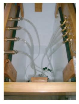
internal setup with all facets and hoses installed. I initially mounted the temp control probe to the freezer wall, but that resulted in eronious rweadings, i then moved it to mount on the wood brace.
