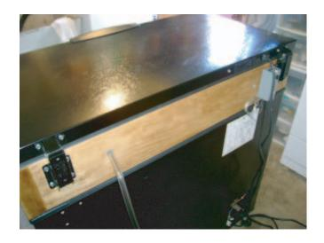
Back view. I chose to keep my CO2 outside to maximize my internal space, since i run up to 4 5gal + 1 3gal kegs and also lager in it. the holes were drilled before the finishing. The temp control is also mounted on the back, and another hole just barely bigger than probe was drilled. They are then sealed with silicone. If you look closely, you can see the splice job I did to extend the cord for the internal lid light. Of course it only works if the kegerator is running.
