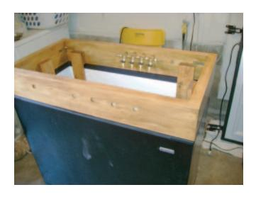
Now it's all fit in and you can see the brass gas manifold (from morebeer) installed. you'll notice i bought a 4-way, but have 5 tap holes, d'oh! Luckily the manifold is expandable.
