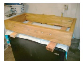
I used a walnut stain (oil based) and covered with 2 coats of oil-based polyeurethane. i only planned on one, but i had runs in it, so ended up sanding the drip marks down and laying on another coat.
